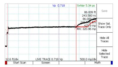
This pin pair shows a much different trace. The cable appears to be broken at about the 86 foot mark. Let's take and save a scan, and then quickly repeat the testing with the other two wire pairs in the cable.
