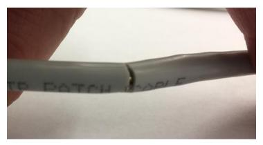
The cut in the cable sliced through two of the individual wires, affecting two of the wire pairs in the cable.
